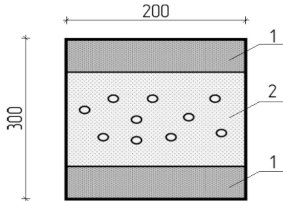
**1 – Layers of Foam Concrete with a Density of  $500 \text{ kg/m}^3$ ,
