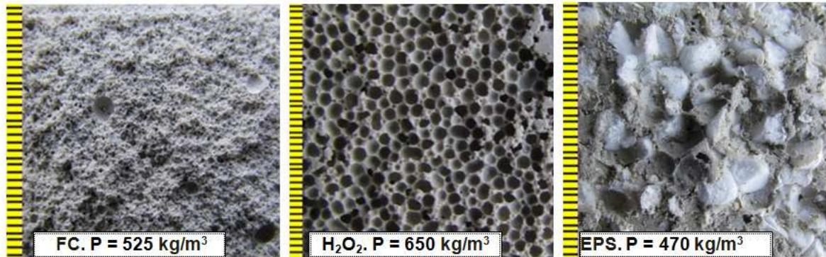
Figure 1: The Impact of the Type of Blowing Agent on Composites Structure
