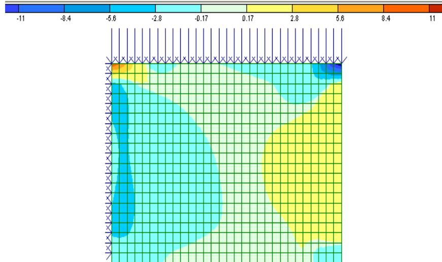
**Figure 9: Mosaic Stress on  $T_{yz}$ ,  $t/m^2$**
