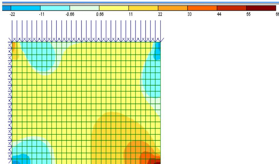
Figure 8: Mosaic Stress on  $T_{xy}$ ,  $t/m^2$
